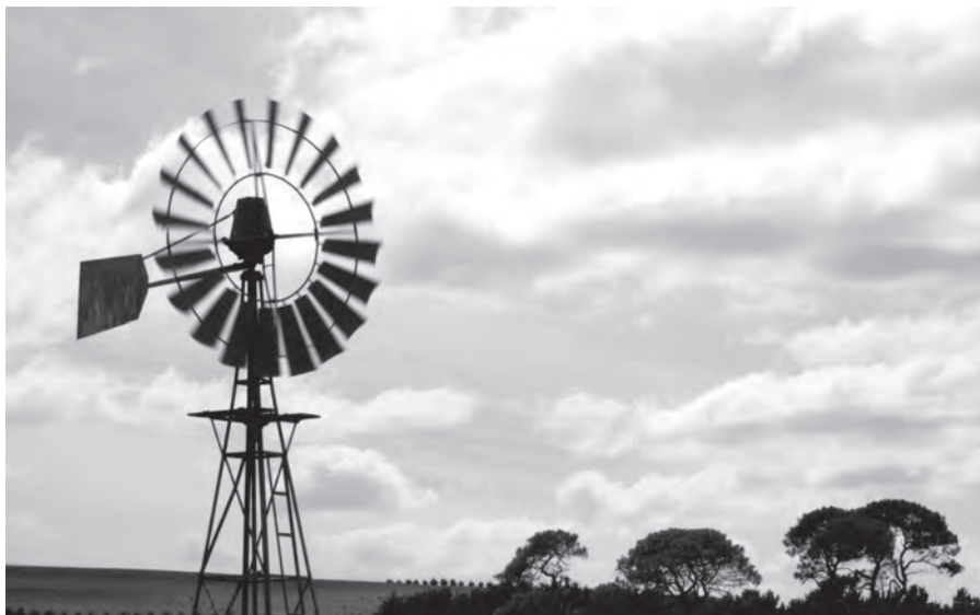
Windmill used for the extraction of groundwater
