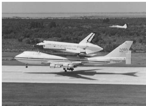
This specially modified 747 is returning the space shuttle to Florida with a piggy back ride after it landed in California. Source: NASA
