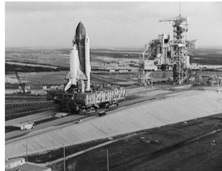
The space shuttle on the crawler, moving towards the launch pad. Source: NASA
