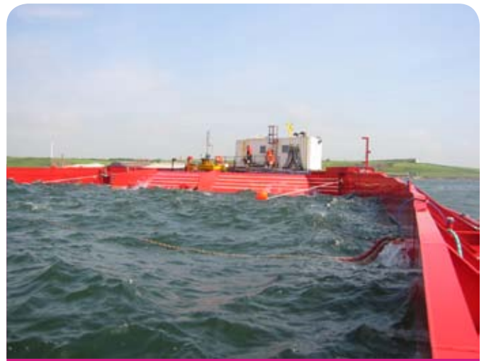
A Wave Dragon wave power facility. This is an example of an overtopping terminator. Source: Erik Friis-Madsen/Wikipedia
