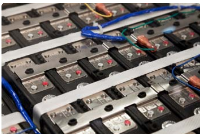
A closeup of an array of batteries inside an electric car. Source: iStockphoto
