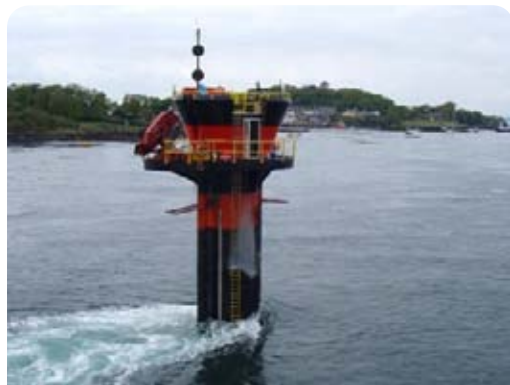
SeaGen - world's first commercial tidal generator in Strangford Lough Northern Ireland. The strong wake shows the power in the tidal current. Source: Fundy/Wikimedia Commons
