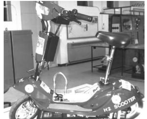
Hydrogen scooter. Source: Hydro Tasmania
