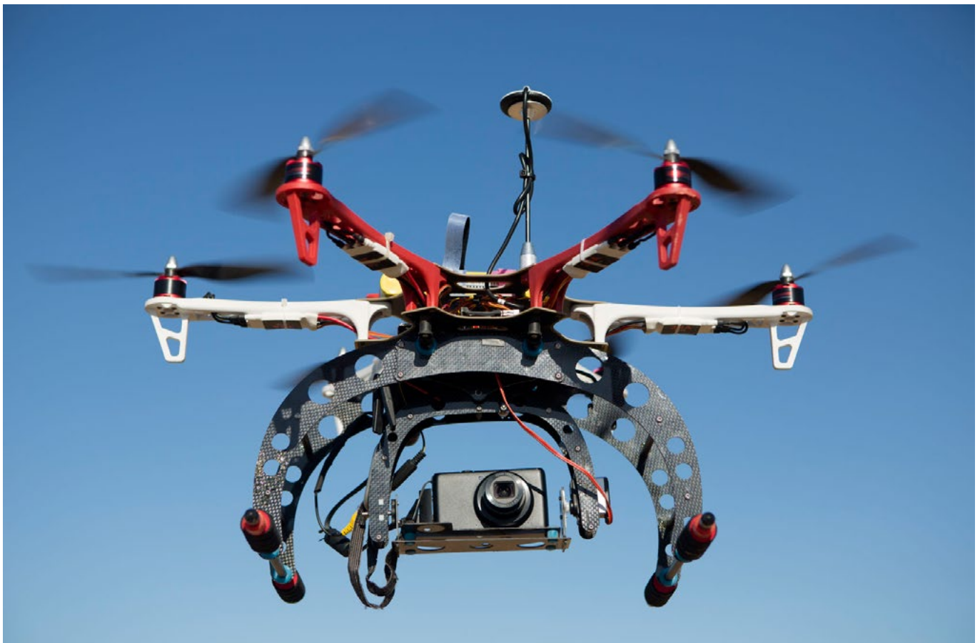
▲ A drone used for aerial photography (Source ©jarp5/123rf)
