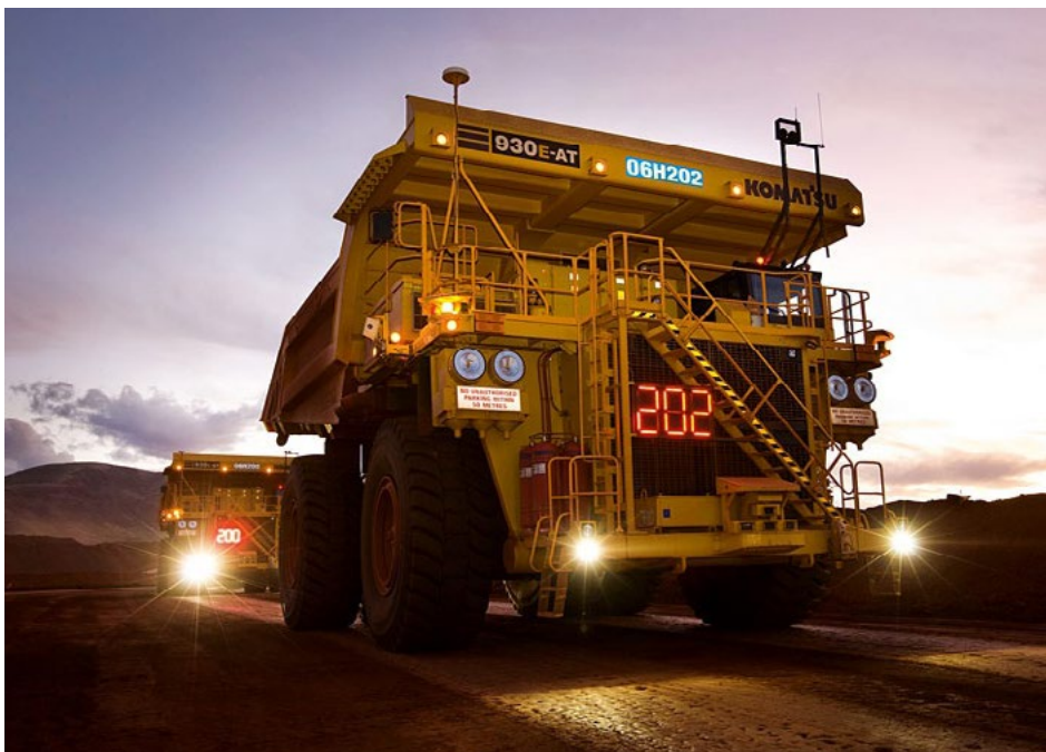
◀ Autonomous Haulage System trucks at the West Angelas mine, WA [Source: M2M ]
