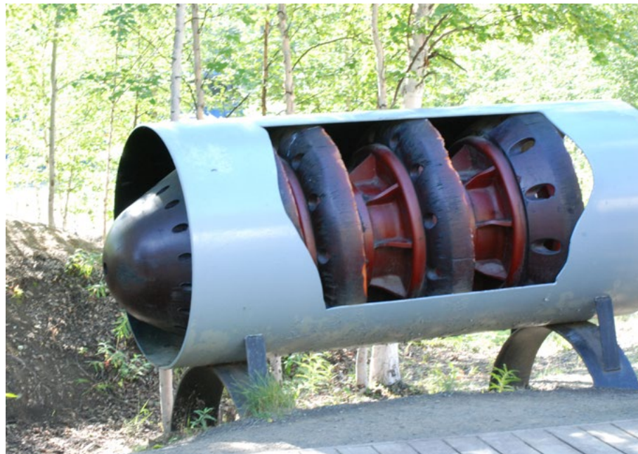
▼ Pipeline pig (Source: Wikipedia, Harvey Barrison, CC BY SA 2.0 )
