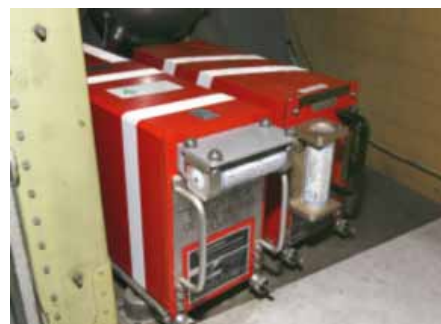
The digital flight data recorder and cockpit voice recorder (black boxes) developed by Dr Warren, Melbourne. Loui Seselja, National Library of Australia, nl39475g-ls1 18
